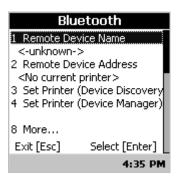
2 Select **Set Printer (Device Discovery)** to start the Bluetooth device discovery. A list of discovered devices appears in the Devices dialog box.
